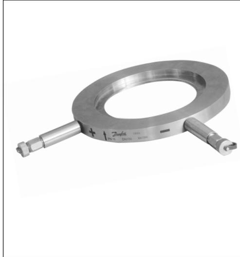
Danfoss flow measuring orifices are used to precisely determine the flow in water based heating, cooling or potable water systems. This determination is done by measuring the differential pressure across the fixed orifice, which has a well known Kv value.
