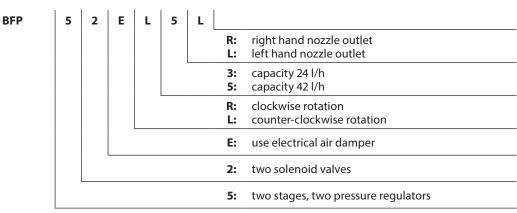
Nozzle capacity at 4.3 cSt., 10 bar, 2800 min<sup>-1</sup>
