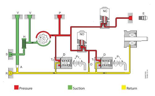
From the suction inlet (S) oil is drawn through the filter (H) to the gear set, where the pressure is increased. By means of the diaphragm (D) in the pressure regulator for stage 1 ( $T_1$ ), the pressure is kept constant at the value set on adjustment screw ( $P_1$ ).
