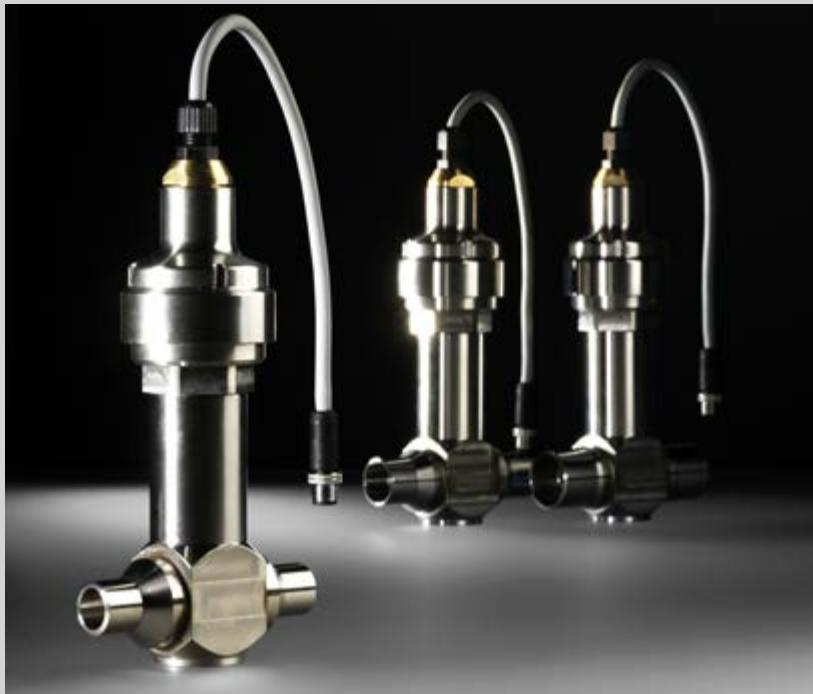
The CCM is an electrically operated valve designed specifically for operation in CO<sub>2</sub> systems. The valve is capable of functioning both as an expansion valve, and as a gas bypass valve with back-pressure regulation in subcritical applications.
