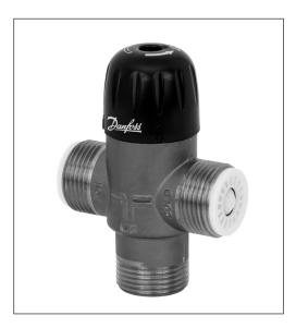
The TVM-W is a self-acting mixing valve, which provides mixed water at a constant temperature. It is used for instant supply of water at a required temperature in domestic hot water applications.
