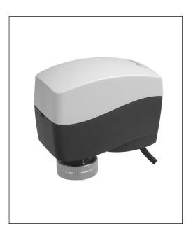
AMI 140 is 2 point 3 wires actuator used with AB-QM (DN 10-32) and VZ, VZL, VRBZ valves. The actuator can be used with fan coil units, induction units, small re-heaters, re-coolers and zone applications in which hot/cold water is the controlled medium. The actuator provides with factory default setting (actuators spindle fully stem up):
