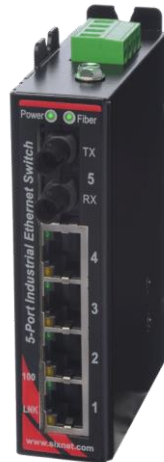
Typical ST style connector on a SLX-5MS-4/5ST
