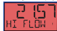
Meter in alarm condition. Display turns red, flashes and shows HI FLOW alarm message.
