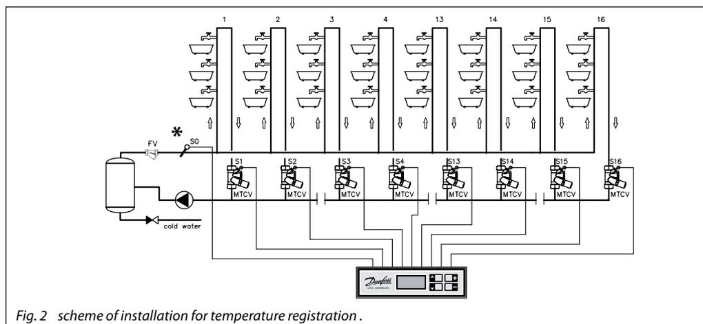
Fig. 2 scheme of installation for temperature registration.
