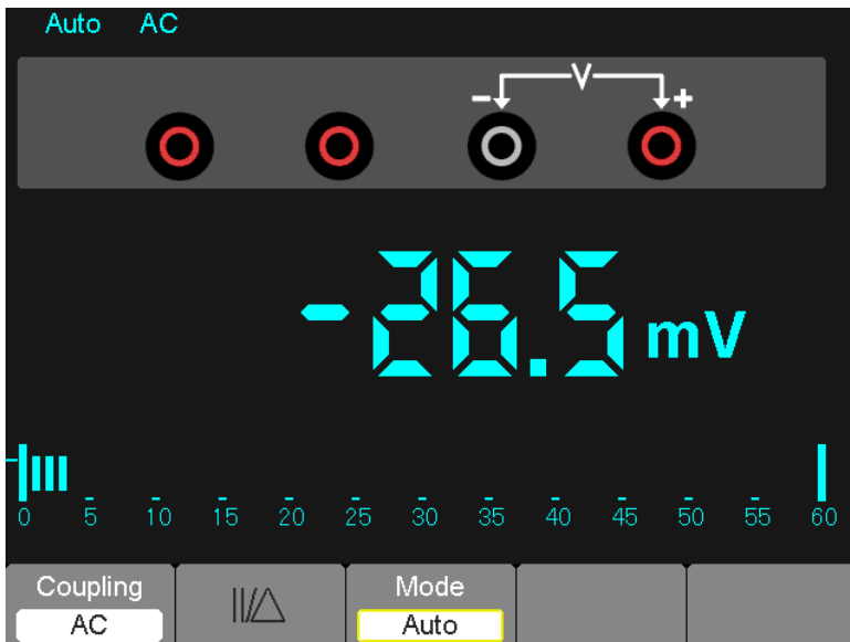
Figure 7-7 AC voltage Measurement
